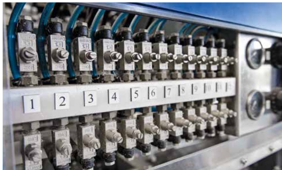
Support air control for the extrusion head
