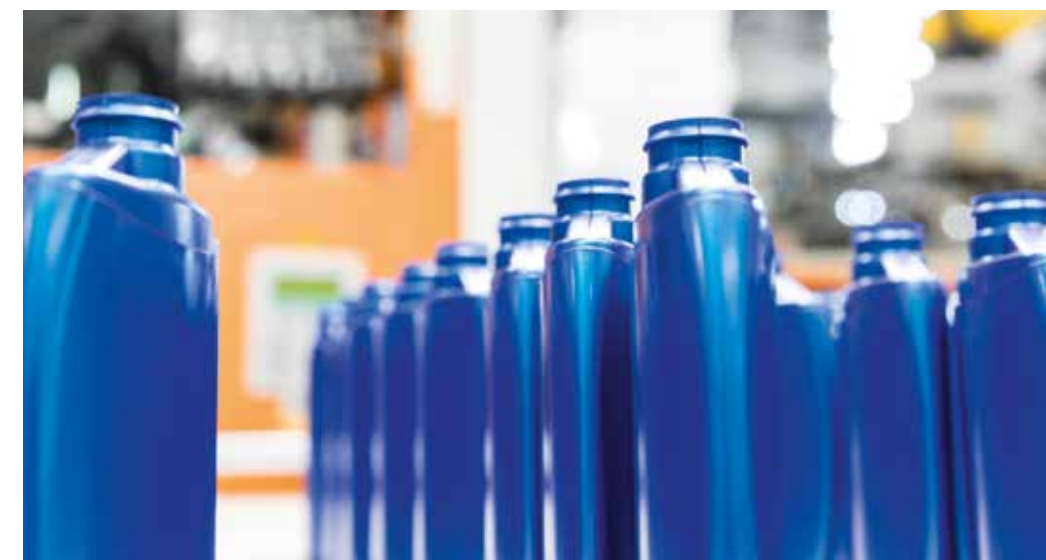
Row after row of finished plastic bottles emerging from the extrusion blow moulding machine
