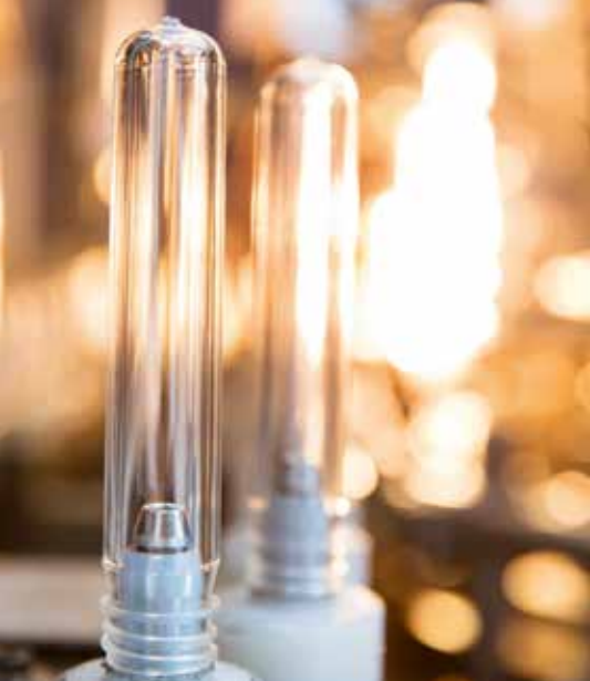
In injection stretch blow moulding, the first step is the pre-form...
